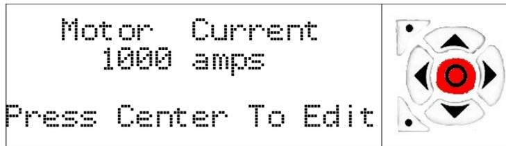
Once in edit mode, the maximum available current will be displayed. The selected digit will show a flashing cursor. Editing can only be done when the controller is not in drive mode. A message will be displayed specifying this restriction if an attempt is made to change the value when in drive mode. To change the value, use the top and bottom buttons. To navigate to the next digit, use either the left or the right buttons.
