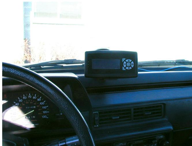
*Illustration 2: Example of IM installation in a vehicle*
