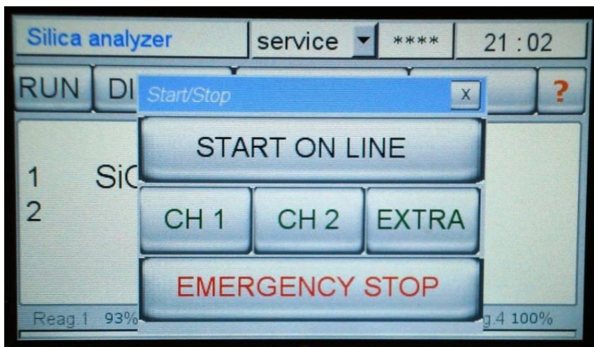
Figure 5.3: User interface after pressing the RUN Menu.
