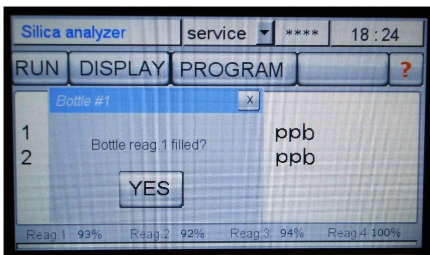
Figure 5.2: User interface screen for Reagents Refill.
