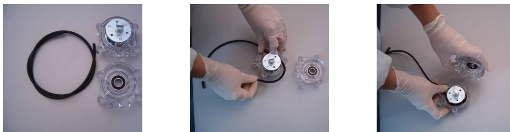
Figure 7.1: Pump tubing replacement.
