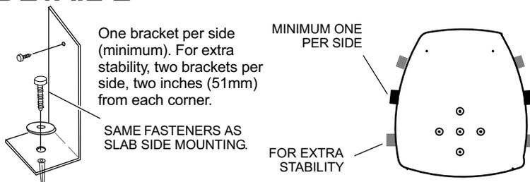
Figure 6. Placement, Slab Mounting and Stabilizing Unit
