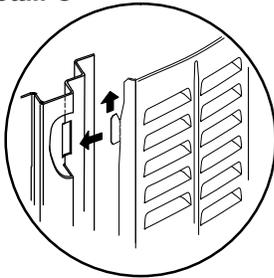
MAINTAIN MINIMUM PANEL ANGLE (AS CLOSE TO PARALLEL WITH THE UNIT AS POSSIBLE) WHILE INSTALLING PANEL.
