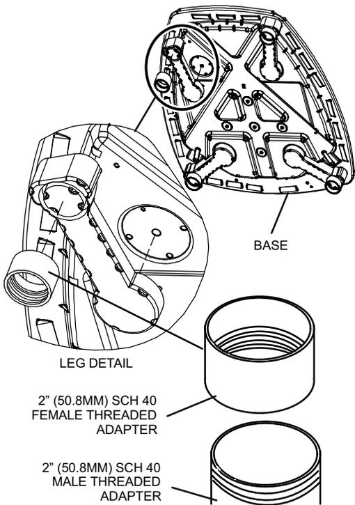
Use additional 2" SCH 40 male threaded adapters which can be threaded into the female threaded adapters to make additional adjustments to the level of the unit.
