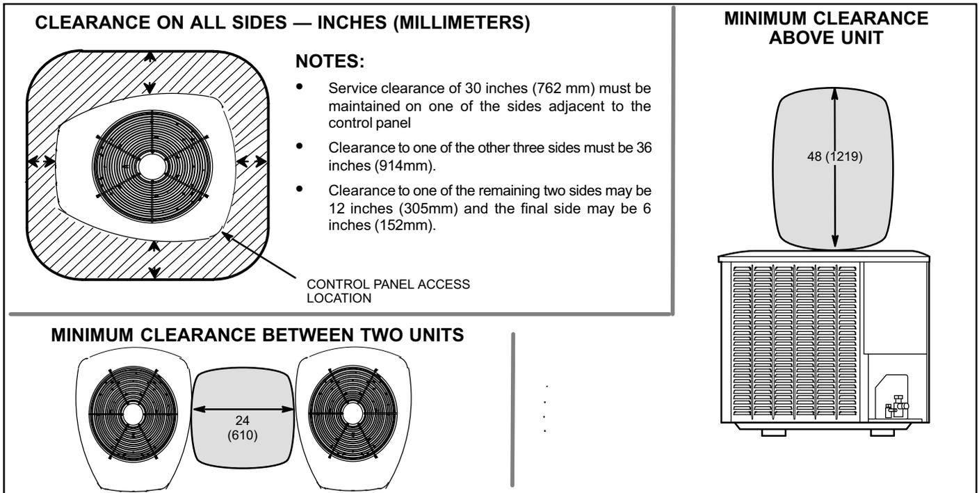
Figure 5. Installation Clearances
