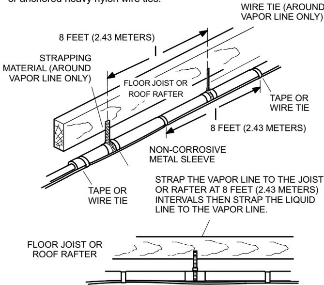
**REFRIGERANT LINE SET — INSTALLING VERTICAL RUNS (NEW CONSTRUCTION SHOWN)**
