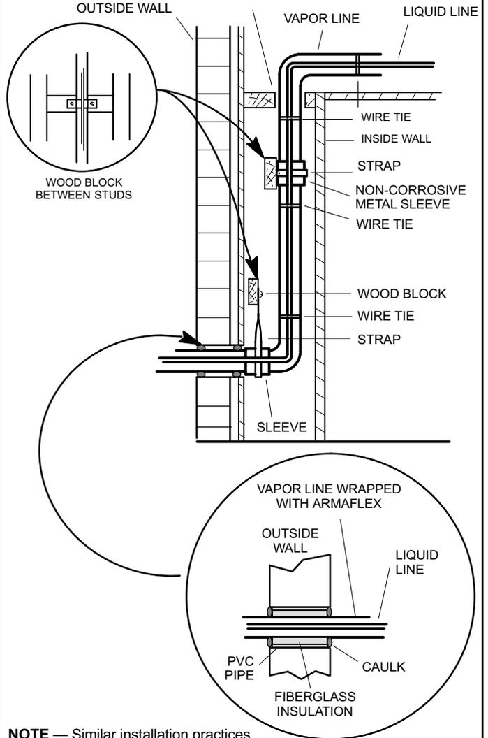
NOTE — Similar installation practices should be used if line set is to be installed on exterior of outside wall.
