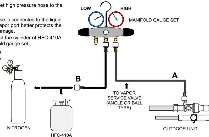
Figure 13. Manifold Gauge Set Connections for Leak Testing
