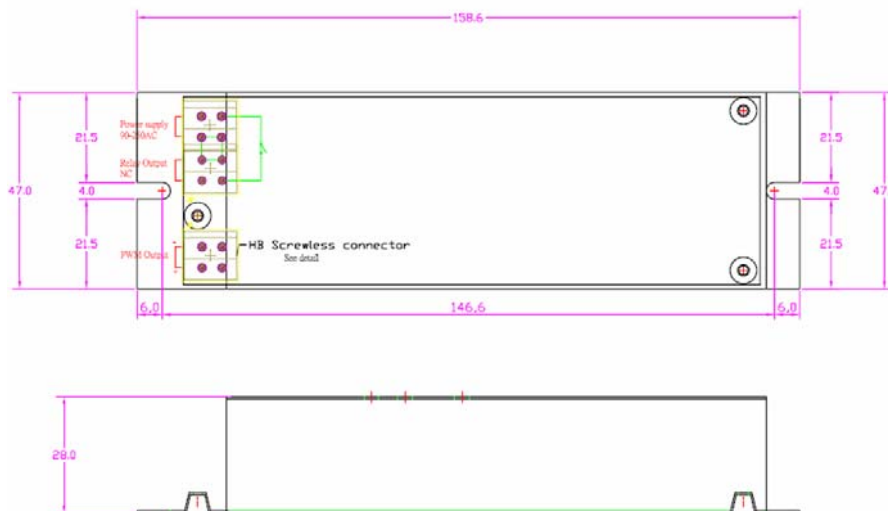
Figure 3.5 Device dimensions without plug-screw clamps
