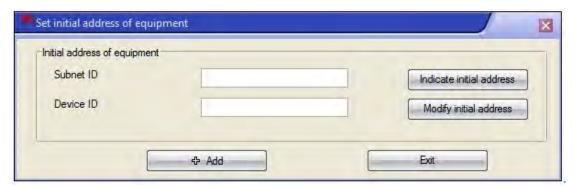
d) Click on "Indicate initial address", and the current subnet/device ID of the device will then be displayed. To modify the address, fill in the new address, and click the "Modify initial address" then click the "+Add" button. The device will now be added to the "ON-line devices list".
