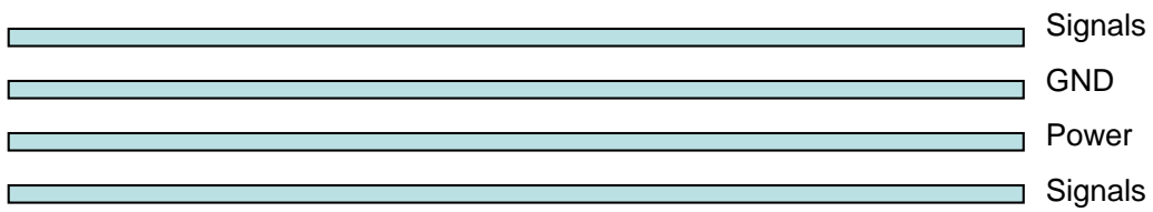
Figure 12: Typical 4-layer PCB construction
