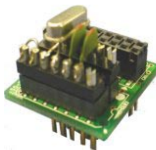
Figure 4-31. Appearance After Mounting Oscillator
