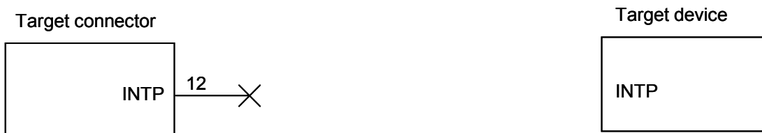
Figure 5-8. Circuit Connection for the Case Where MINICUBE2 Is Used Only for Programming
