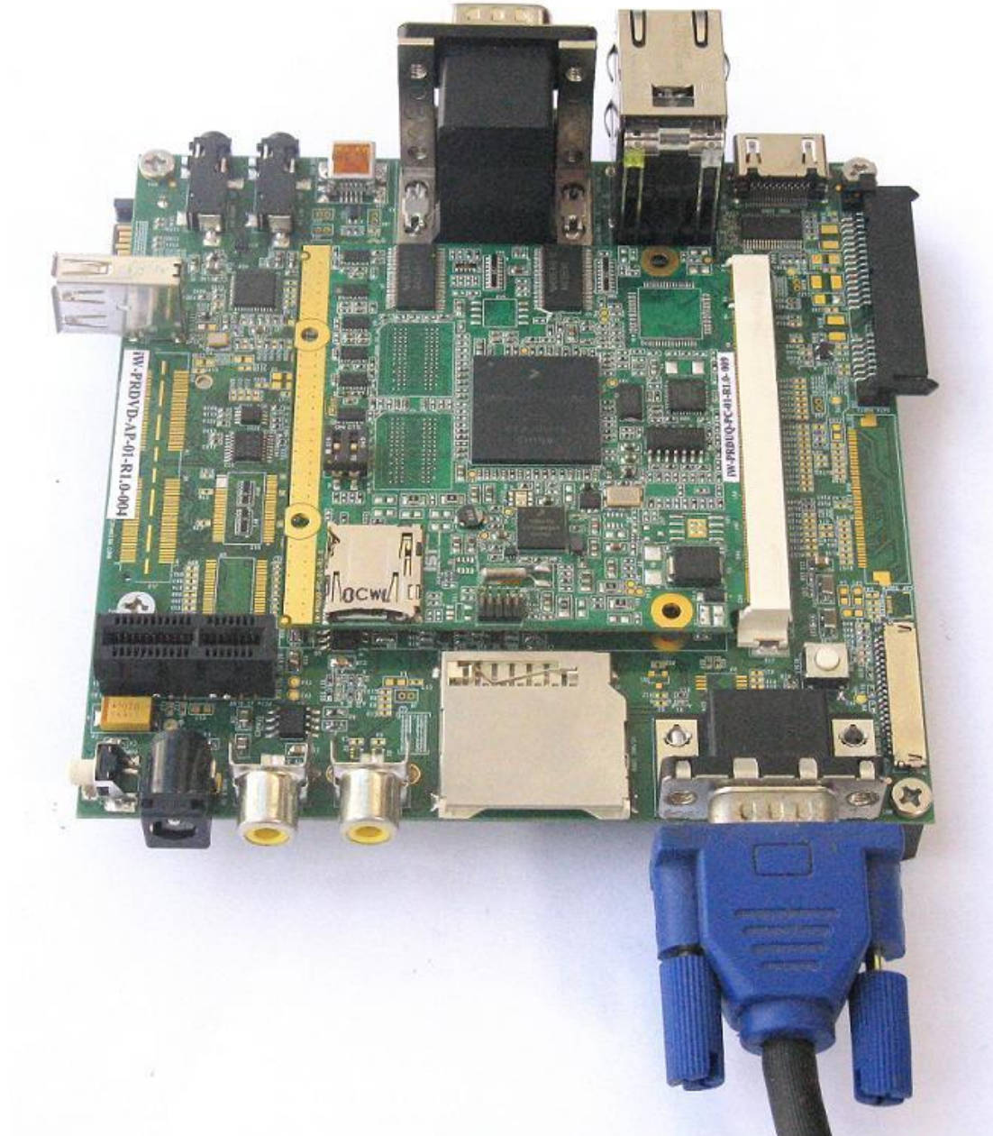
Figure 10: VGA Cable Connection
