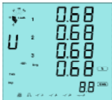
Fig 3.14 THD of phase voltage
