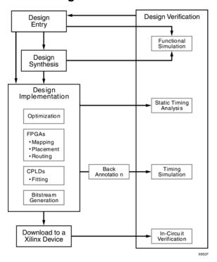
The following figure shows the Xilinx software flow chart for FPGA designs.
