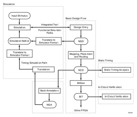
The following figure shows the verification methods of the design flow for CPLDs.
