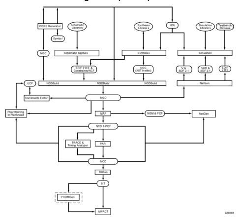
The following figure shows the Xilinx software flow chart for CPLD designs.
