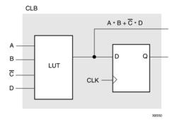
Observe that MAP has generated an active low (C) instead of an active high (C). Consequently, the Boolean output for the combinatorial logic is incorrect. When you run NetGen using the mapped.ngm file, you cannot detect the logical error because the delays are back-annotated to the correct logical design, and not to the physical design.
