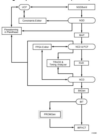
The following figure shows the design implementation process for CPLD designs:
