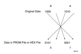
In a bitstream contained in a BIT file, the Least Significant Bit (LSB) is always on the left side of a byte. But when a PROM programmer or a microprocessor reads a data byte, it identifies the LSB on the right side of the byte. In order for the PROM programmer or microprocessor to read the bitstream correctly, the bits in each byte must first be swapped so they are read in the correct order.
