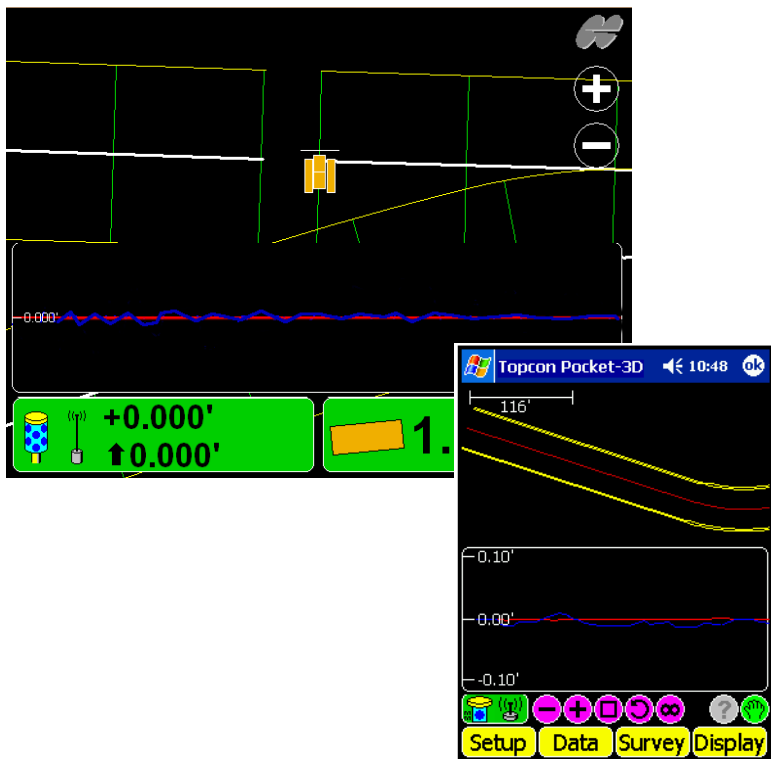
Figure 7-24. Cut/fill History Windows for 3DMC and Pocket-3D
