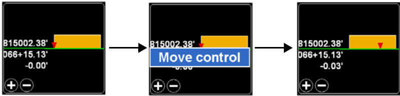
Figure 8-22. Move Blade Control Point Using Section View
