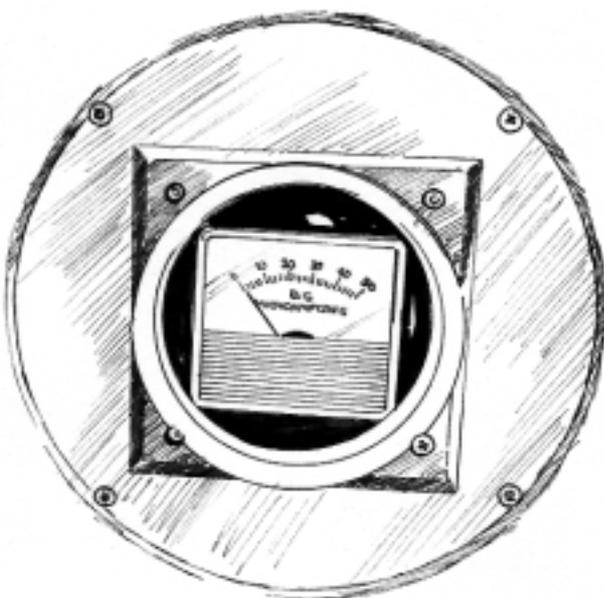
**Diagram 8:** Gauge showing that the probe is not in the water
