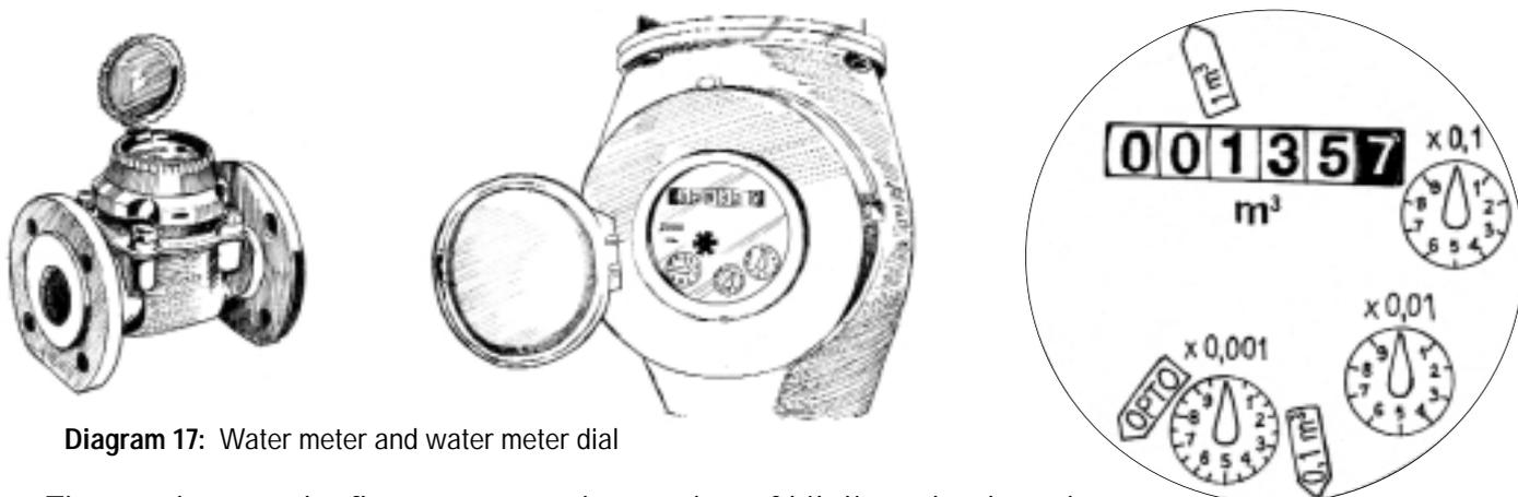
Diagram 17: Water meter and water meter dial
