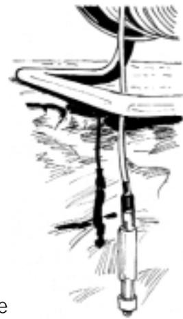
Diagram 6: The dip meter probe
