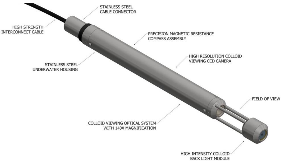
Figure 1.1 –Colloidal Borescope Probe Features
