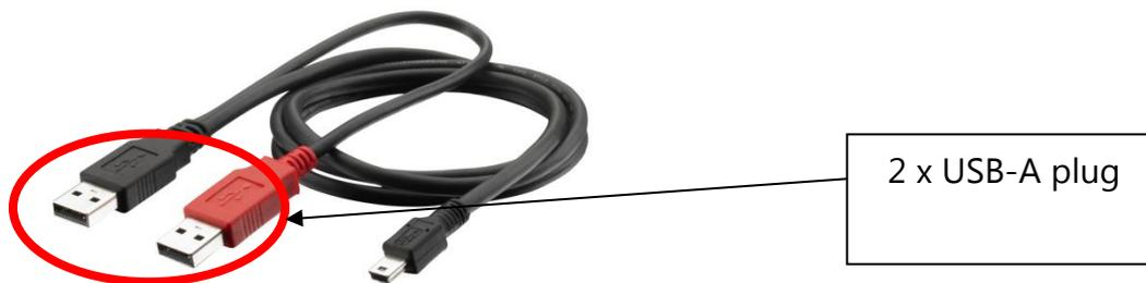
Second, connect the other end of the cable (mini-USB) to the USB2DALI interface.
