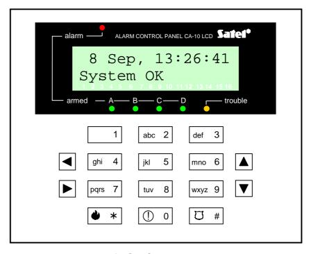
Figure 1. View of LCD-S keypad.
