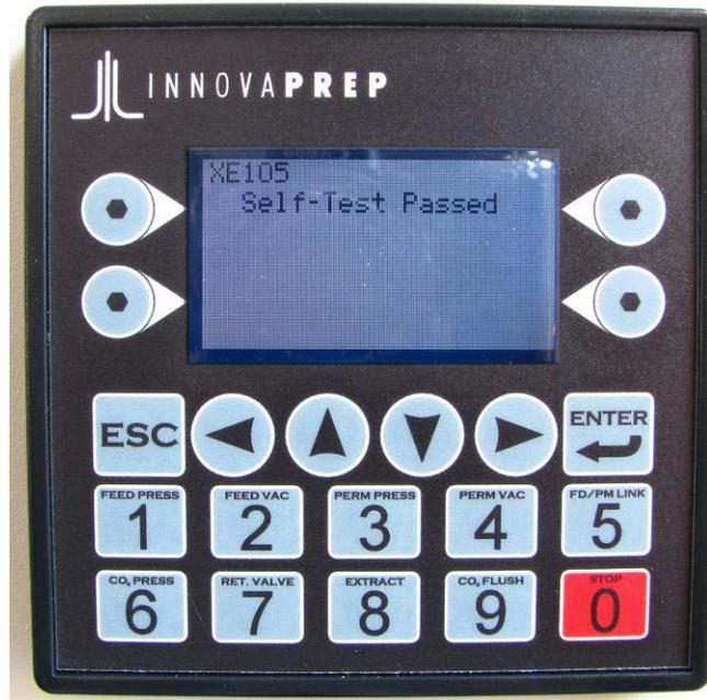
Figure 4-2. Controller Self-test Passed
