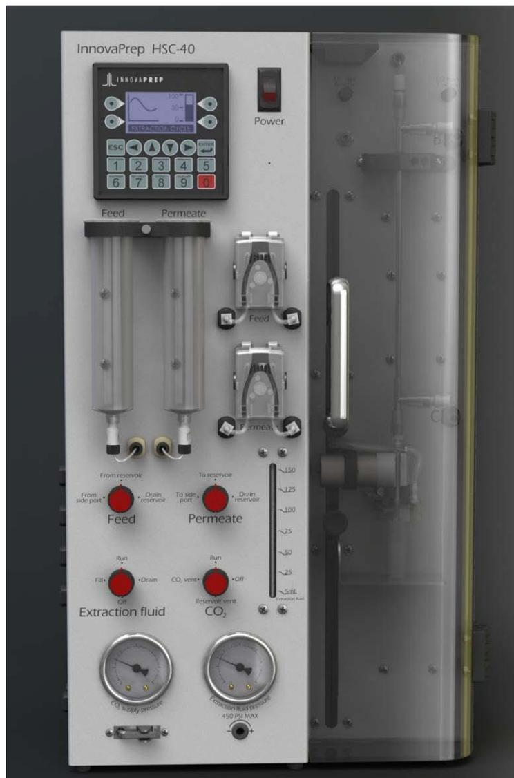
**Figure 2-1. InnovaPrep Model HSC-40 Front Panel**
