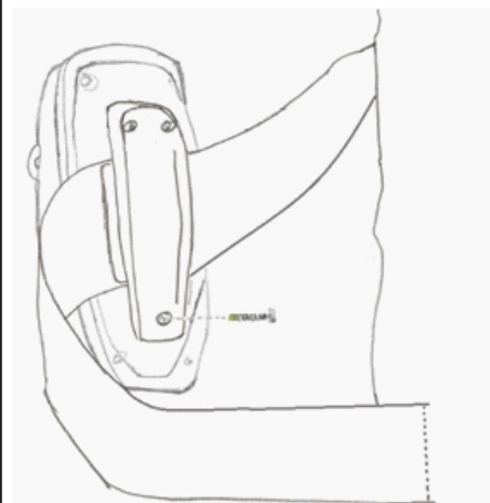
Position of the beacon on the inflated life jacket
