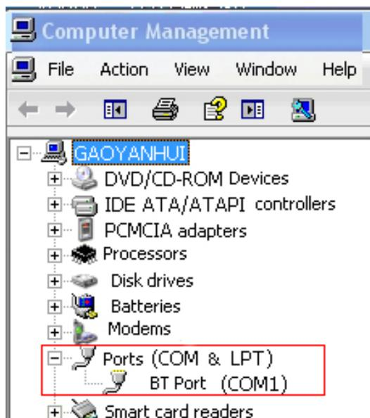
Remember the COM you are using and then run the control software, find **【Communication】** option, Click Com button, buttons will turn green. As following:
