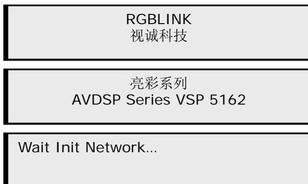
VSP 5162 can be connected via network cable to the LAN, but when the device is not connected to the network, there will be a prompt: DHCP Failed; The device does not show DHCP Failed when you access the network: as following:
