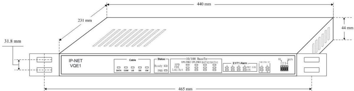
Fig.3.1-1 Mechanical dimensions
