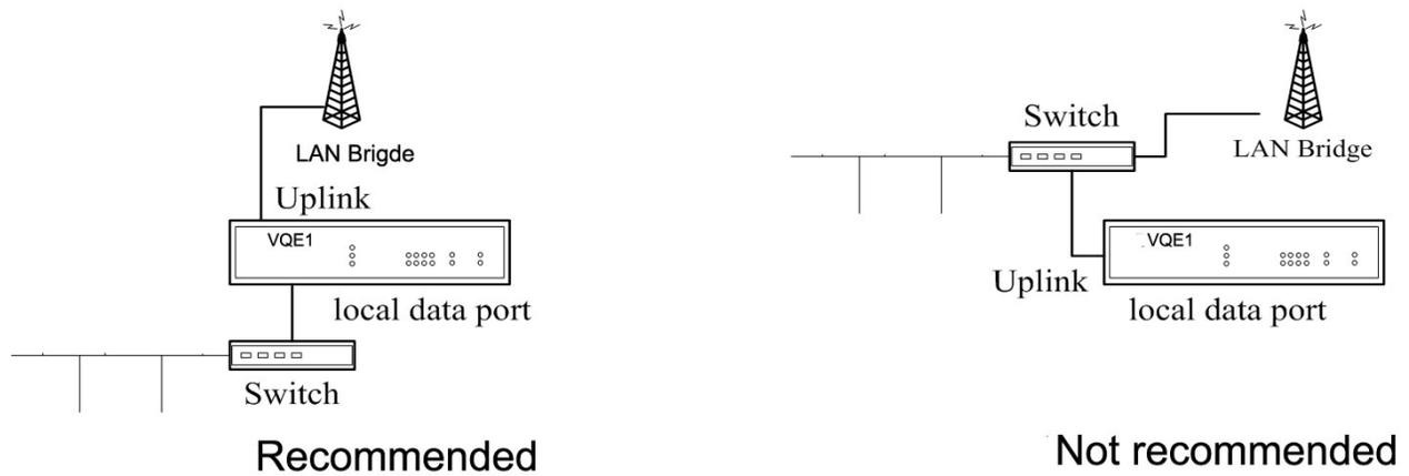
Fig. 1.3-2 Preferred connections for LAN traffic
