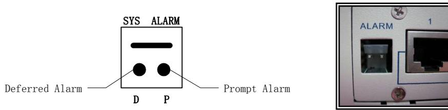
Fig. 2.4-2 System alarm port
