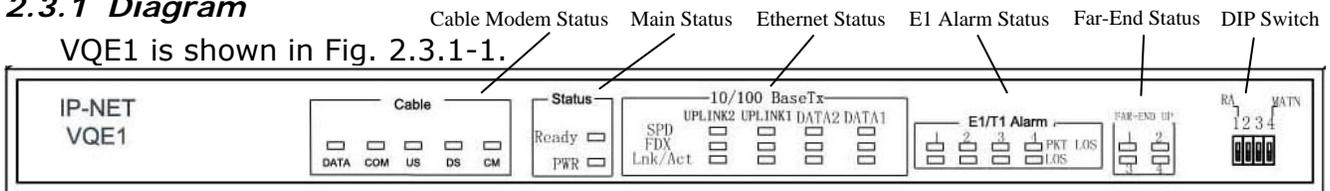
Fig. 2.3.1-1 Front panel of VQE1
