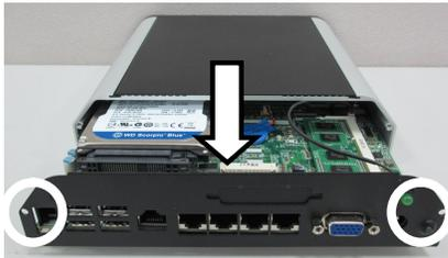
2. Remove the I/O cover screws (x2) and slide out the I/O cover.
