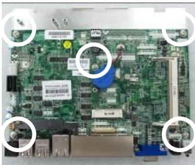
4. Remove the screws (x5) on the Motherboard.
