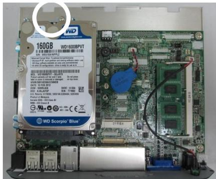
3. Remove the HDD screws (x3).
