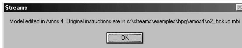
This message is obtained whether the model has actually been changed or not. The instructions from which the original Amos Graphics model was created are kept unchanged in the file name given in the message box. Should the changes made in Amos Graphics not be wanted, or incorrectly interpreted by STREAMS, the original instructions may easily be brought up again, just through opening the model.
