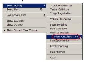
The F5 key allows the user to launch a "silent dose calculation" when it is unnecessary to modify the default dose calculation parameters (dose calculation algorithm, inhomogeneity correction). In this case, the Options dialog window of the Dose Calculation activity (that includes the external extension values) is not displayed and the calculation job is sent to the calculation queue.
