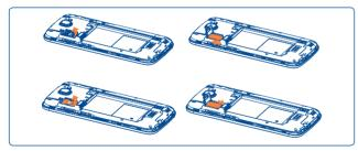
To install, please start by sliding the metal Micro-SIM card tray to up unlock position, the tray will click and release when unlocked. Place the Micro-SIM card into the slot with the gold contacts facing downward. Once SIM card is placed into slot, close metal SIM card tray, then slide tray to down lock position, tray will click when locked.
