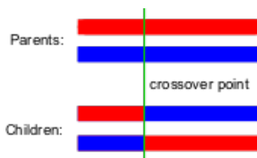
Figure 1: An example of one point crossover, obtained from http://en.wikipedia.org/wiki/Crossover_(genetic_algorithm)
