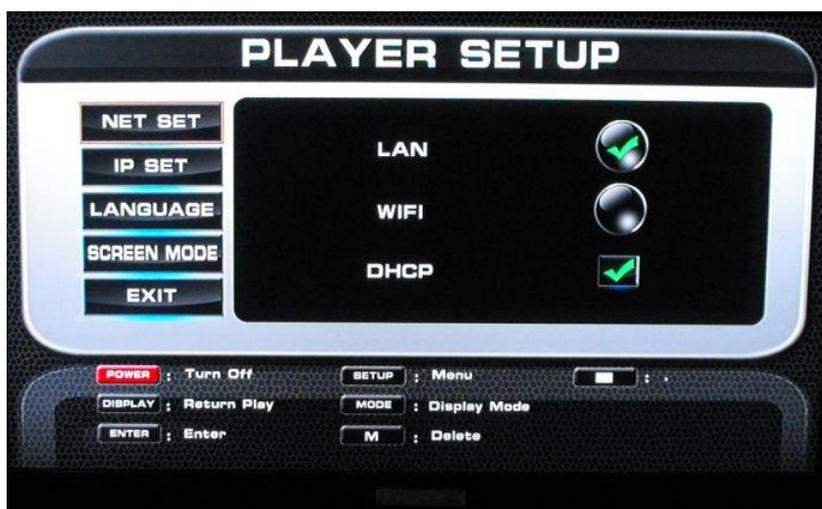
2.start the network setting of information in interface, include IP address,subnet mask,gateway,and server(IP、 Mask、 Gway 、 Server). .That is to say,when use wire LAN,you must write the first four lines
