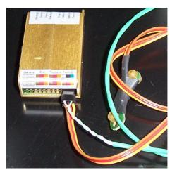
Connect the throttle lead from the RX in its place, in the upper position. Lower socket is ready for a second servo signal but not used on present firmware
