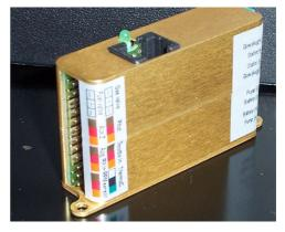
Connect the RPM sensor and thermocouple on its respective sockets, in the orientation that is shown in the colored labels on the fadec. If necessary both leads can be extended using good quality servo extensions.
