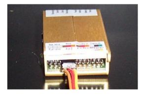
The last two sockets are used for the connection of the solenoid valves. Upper position for the gas/keroburner solenoid and the lower position (as shown in the picture) for the main fuel valve.
