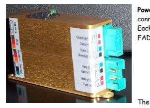
**Power connections:** Two high quality MPX connectors carry all the power current. Each power lead is identified by the label on the
