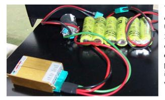
The lower MPX plug provide the connection to the pump and the battery. Use 0,5mm cooper lead for the pump and 1mm for the battery. Keep all connections well isolated between them, and be sure to not reverse the battery polarity, the fadec will be burned out immediately. The battery minimum voltage is 7,2V and maximum 8,4V.
