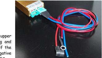
MPX plug provides the power to the glow plug and starter motor. Use 0,5mm flexible cooper lead if the length is up to 0,5m, and 1mm if higher. Both negative leads are connected to same place inside the FADEC, so
