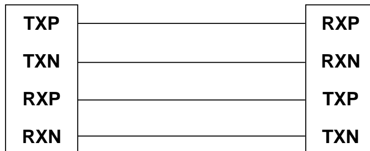
Figure 2.2.2.1-1 NMEA 0183 to RS-422 Connection
