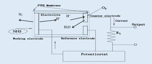
The NE4-NH3 consists of 3 porous noble metal electrodes separated by an acidic aqueous electrolyte, housed within a plastic (PPO) enclosure. Gas enters the cell via a gas phase diffusion barrier. An electrolyte reservoir ensures an excess of electrolyte is available at all times, and the sensor is vented to ensure that the internal and external pressure of the sensor is always in equilibrium.
