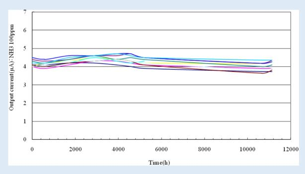
This data was generated in bench tests in a controlled clean environment. In service, in a real application, the long term stability will also be dependent on the environmental conditions of the application.
