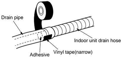
**F Wrap the insulation material around the connecting portion.**
