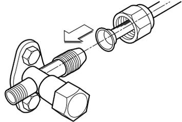
**C** Finally, tighten the flare nut with torque wrench until the wrench clicks.
