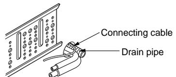
**C** Insert the connecting cable into the indoor unit.
