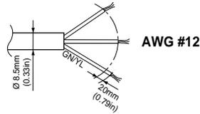
The connecting cable connected to the indoor and outdoor unit should be complied with the following specifications (UL and CSA recognized one).
