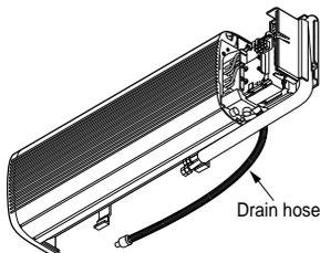
**B** Insert the connecting cable into the indoor unit from the outdoor unit through the piping hole.
