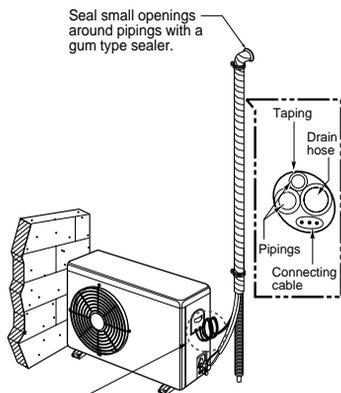
Trap is required to prevent water from entering into electrical parts.
