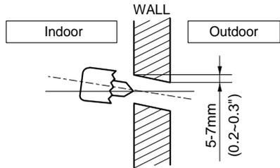
**B** Measure the wall and mark the centerline. It is also important to use caution concerning the location of the installation plate—routing of the wiring to power outlets is through the walls typically. Drilling the hole through the wall for piping connections must be done safely.
