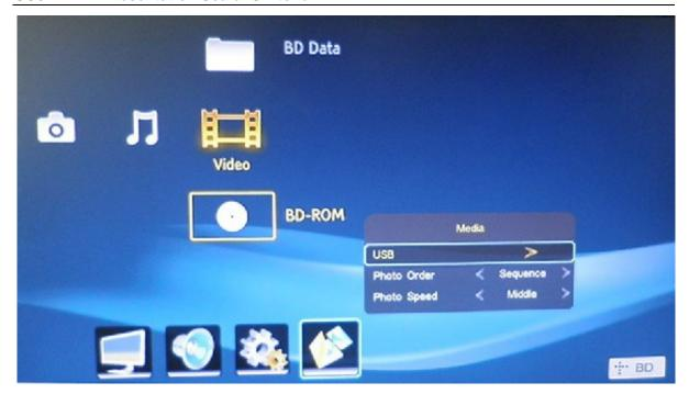
When you enter this page, you can select the file from USB flash disk, which is plugged to SC61D. You can use the up/down/left/right buttons to control it.
