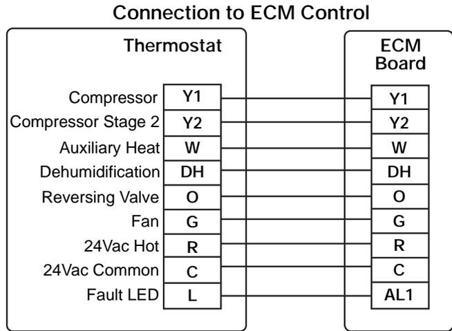
Units with CXM or DXM board and ECM fan motor, utilizing ECM dehumidification mode
