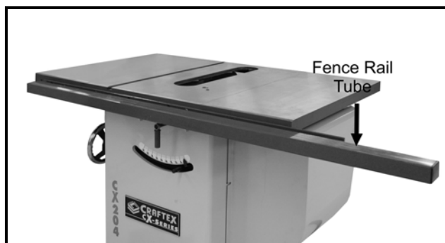
Figure-11 Installing the fence rail tube
