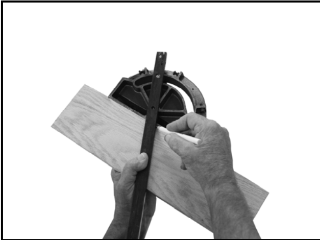
Figure-31 Marking the angle of cut
