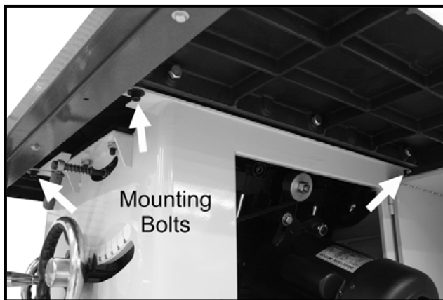
Figure-33 Mounting bolts location
