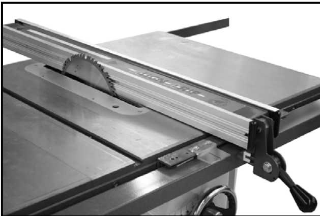
Figure-16 Fence locked on the rails against the blade
