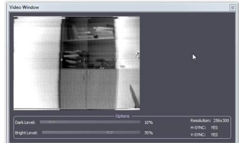
For example, when you select the frequency of the wireless video camera, in the **Video Window** will be displayed black and white image of a television signal.
