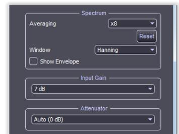
Selecting the type spectral window is a compromise between spectral resolution of adjacent signals, accuracy of the spectral resolution and spectral leakage. Windows are listed in order to improve the spectral resolution and spectral leakage reduction.
