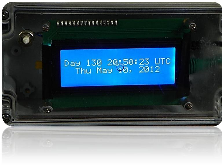
The SNTP Display is based on the #Twatch project by Ian Lesnet, Dangerous Prototypes and is based on the Microchip 18F67J60 microcontroller with full Ethernet support. It's connected to an HD44780-based LCD display with 4 lines of 20 characters. The original #Twatch connects to the Internet to retrieve the top-trending Twitter topics at any moment, and it also has a Matrix Orbital emulation mode to enable applications to use the LCD for display.
