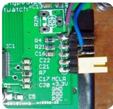
Plug in the #Twatch. The LCD may show garbage or be blank and the backlight will be off.
