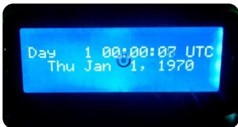
The clock has started but has not gotten sync from the NTP pool. The clock will always start at the Unix epoch time of January 1<sup>st</sup>, 1970, until it connects with an NTP server.
