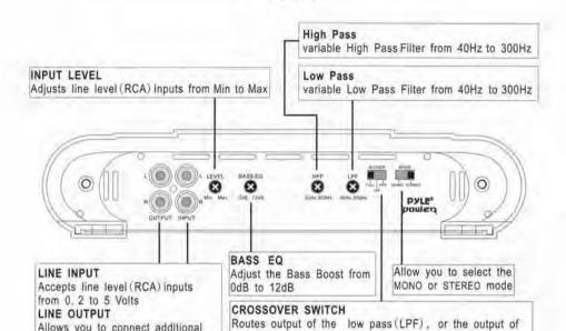
the high pass (HPF) filter, or FULL to the internal power
