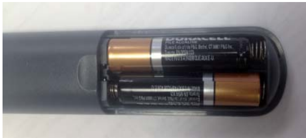
Figure 3: Batteries should go in like this
