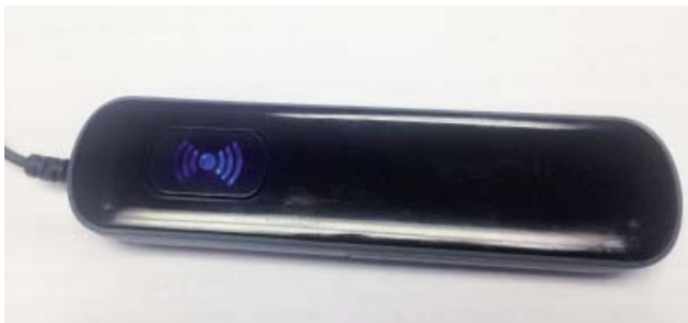
Figure 1: Indicator light indicates status of the GMA. It may appear as blue or red, depending (see next page).
