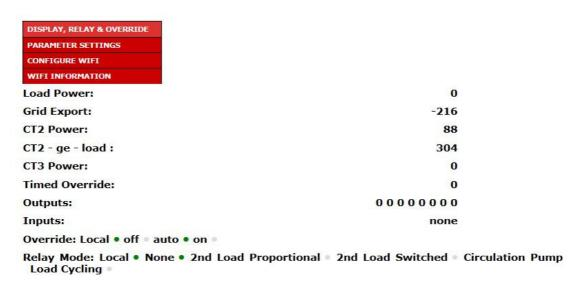
From this can be seen all the four energy flows, the difference between two of them, the status of inputs and outputs, the mode of operation and the front panel switch/relay can be overridden. Data is updated once a second giving a superbly fast view of changes in house loads.
