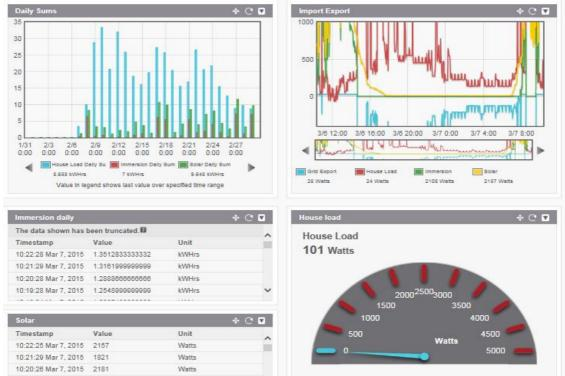
Separate pages enables the user to control the I3 remotely. The I3 is supplied with a range of dials, graphs and tables which the user can configure to suit their needs. Extra dials, etc. can be added and rules set up to trigger events such as "Generation is exceeding 2500W so send me a text and email to remind me to turn on the washing machine". These additions
