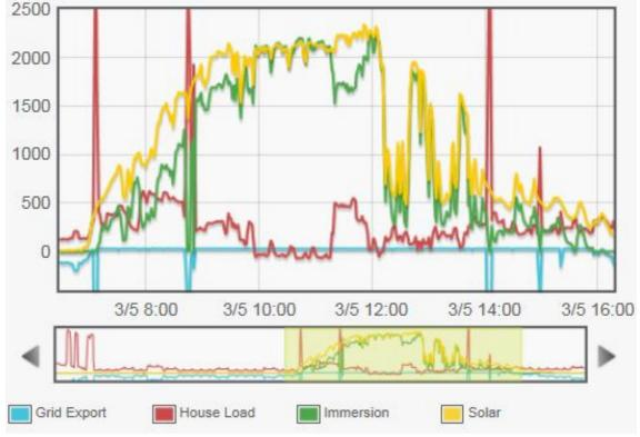
In this case there has been some import when kettles have been boiled (large red spikes) but the immersion was immediately turned off by the I3 during these so no import fed the immersion as seen in this expanded view.
