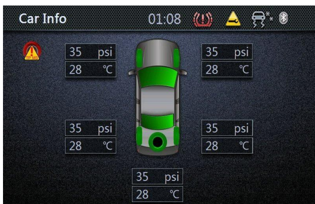
Fig.8. Application for pressure and temperature monitoring system
