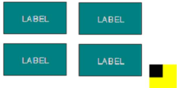
flexibility for cutting. The distance between jobs, the last cut line of the previous frame and the target on the next frame must be between -4 and 4 inches (101 mm). If the distance between frames is less than the scan length, then the target must be outside of the area where the labels are printed. (**Note:** every frame of a label run must be identical or you won't be able to use the copy command). Maximum frame size is 14 inches (35.5 cm) for units shipped after 5-1-10.
