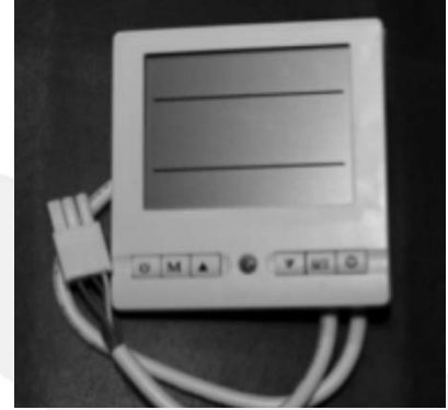
Figure 8-5: ATC control unit
