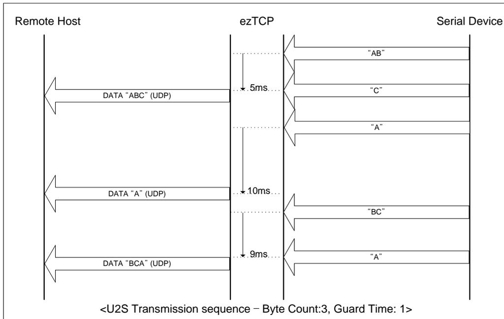
In addition, if the [Peer Address] and [Peer Port] are set to 0, U2S echo functions will be applied. This option allows it to send UDP packets according to the source IP address in the last packet which is received. By using this, CSE-H21 can send multiple hosts one by one. This function is available on 1.2H or subsequently released firmware version.
