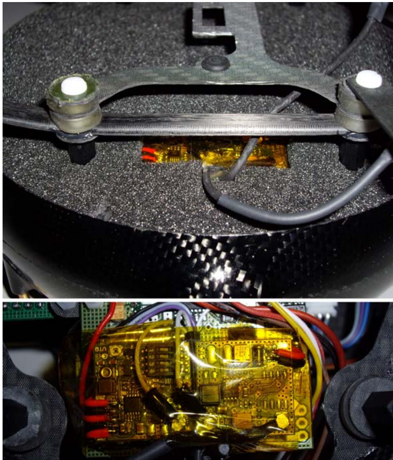
figure 29: video transmitter and booster in the drone
