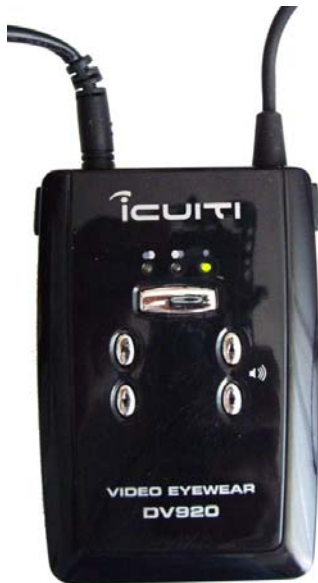
figure 40: control device for the video visor
