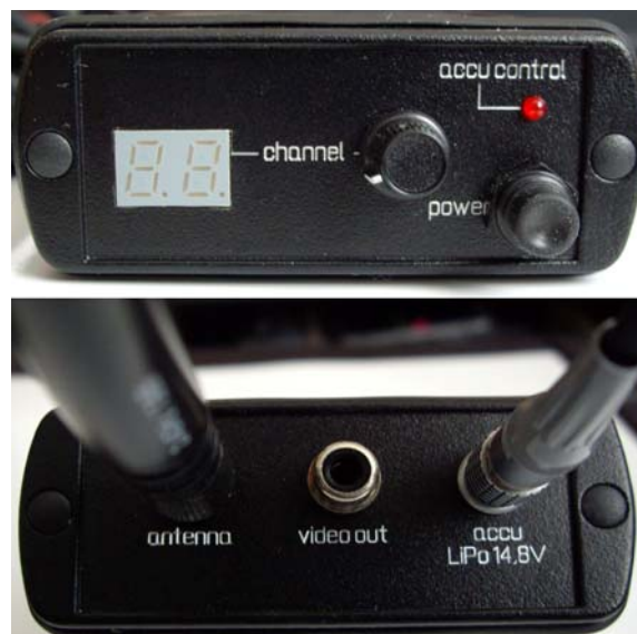
figure 46: control elements of mobile video receiver
