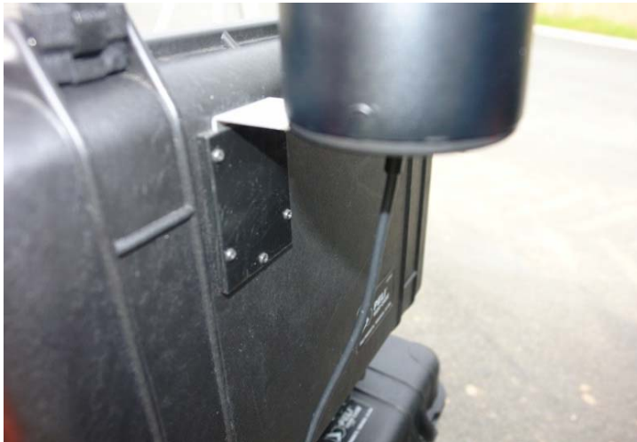
figure 32: mounting the base station antenna
