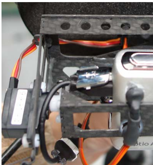
figure 27: connecting the servos for the camera
