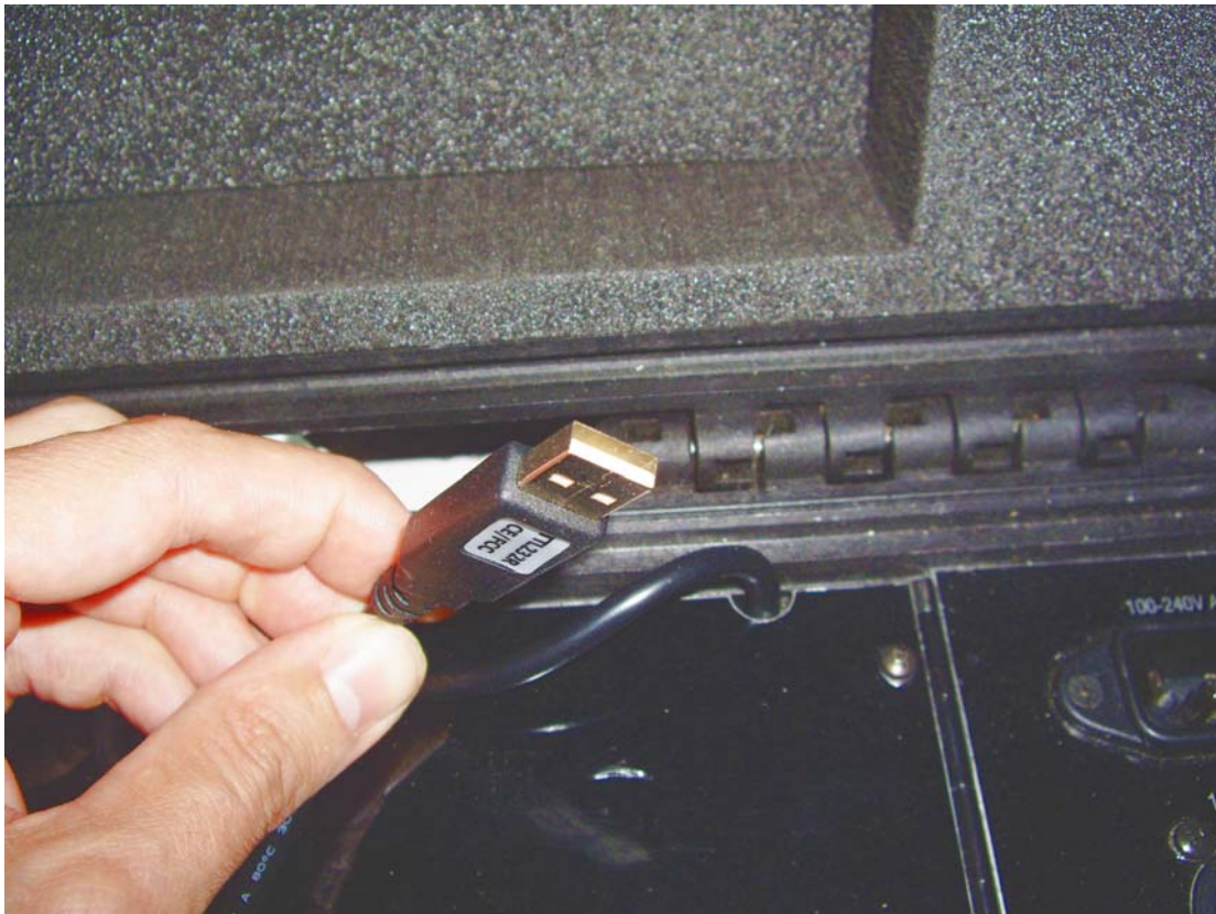
figure 43: USB-connection of the downlink decoder
