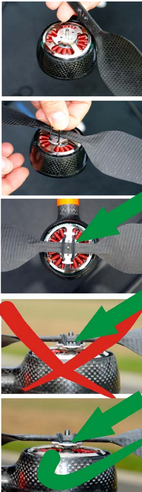
figure 25: mounting the rotor blades
