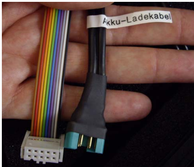
figure 34: connection of the LiPo-charger
