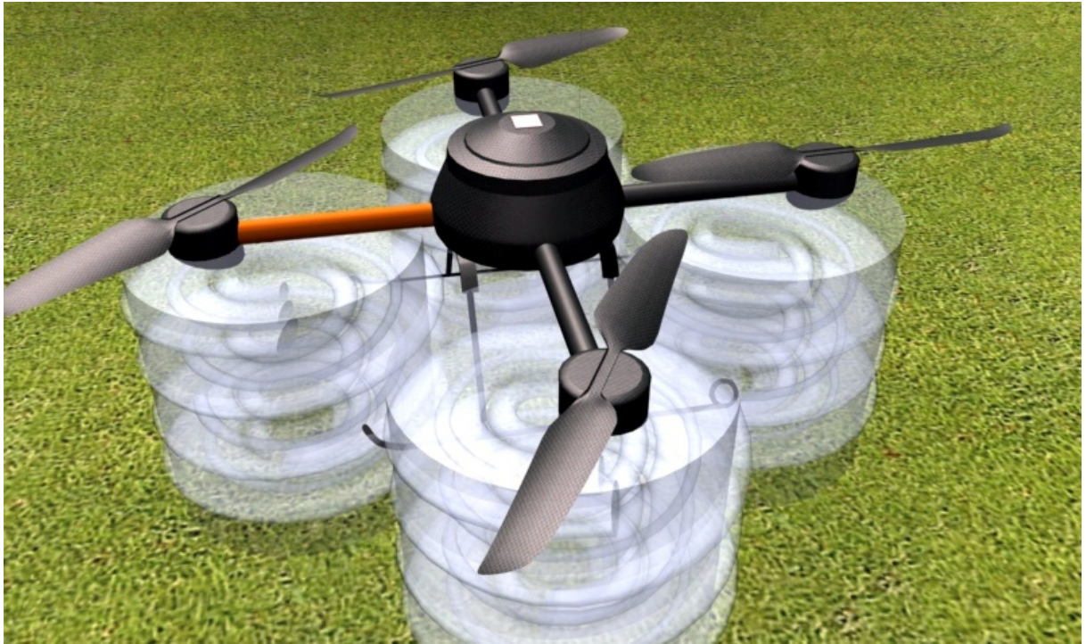
Figure 67: the ground bounce effect
