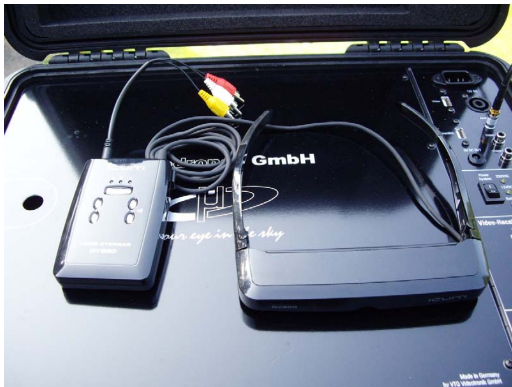
figure 37: components of the video visor
