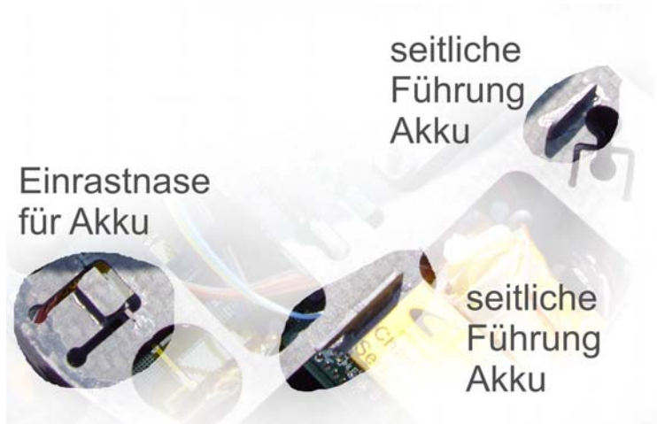
figure 21: support mechanics of the battery pack
