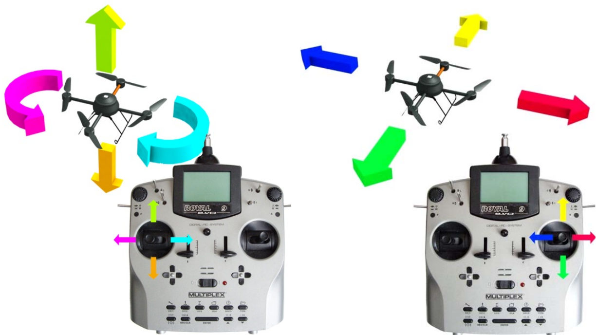
figure 15: assignment of joysticks to movements
