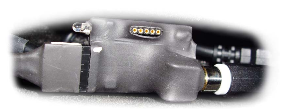
figure 42: downlink decoder mounted
