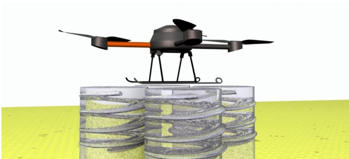
Figure 66: basics of the downwash effect
