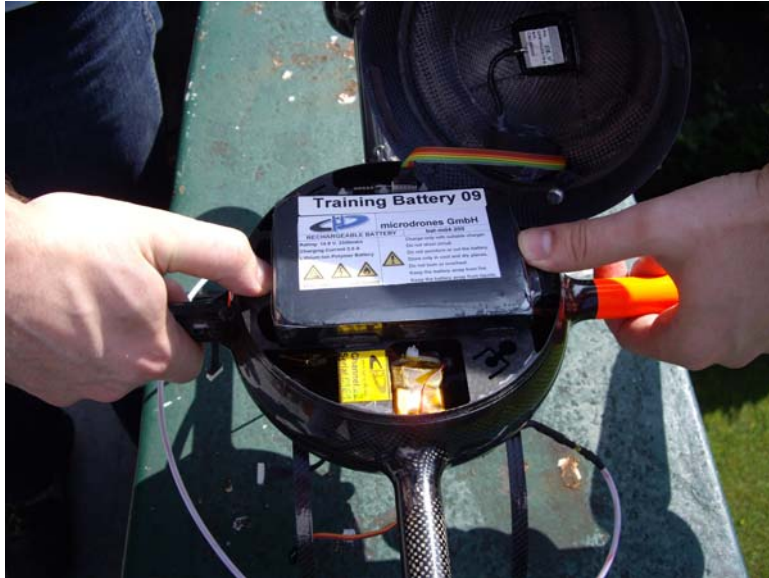
figure 24: unlocking the battery pack
