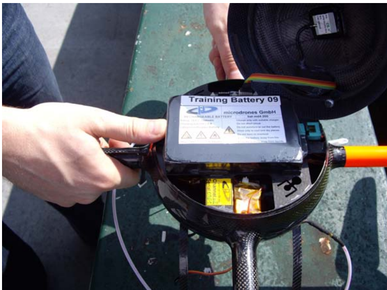
figure 23: inserting the battery pack
