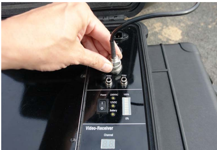
figure 33: connecting the antenna cable
