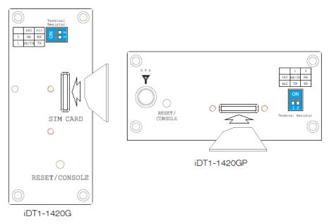
STEP 8: Append SIM cover or DIN-Rail clip to iDT-1420G/GP.
