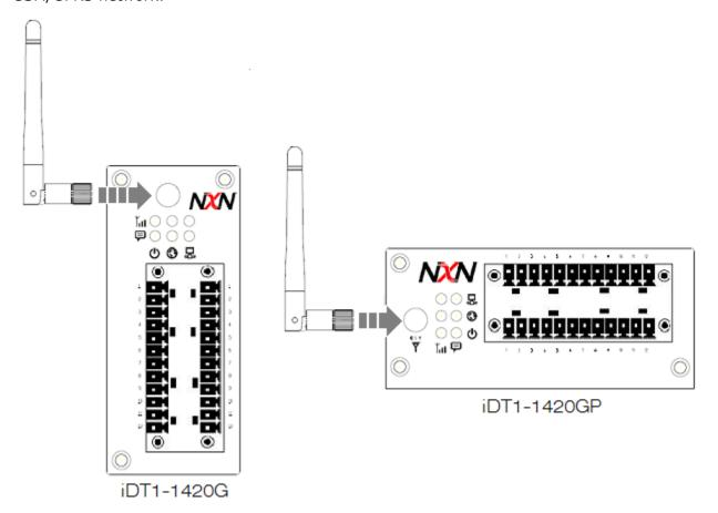
STEP 3: Connect GPS antenna to iDT1-1420GP for receive signal of satellites.
