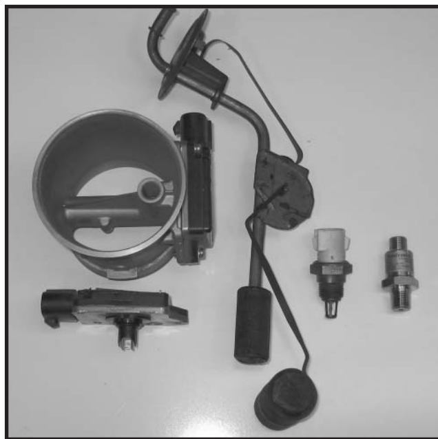
Photo 1 —Here is a sampling of sensors, including a mass airflow housing and a sense element, an MAF element, a fuel level float sensor, air charge temperature, and a Senstronics 0- to 100-PSI pressure sensor. The MAF and temperature sensors provide nonlinear outputs between 0 to 5 V. The pressure sensor produces a 0- to 5-V linear output and the fuel level sensor a semilinear 12- \Omega full/73- \Omega empty output.
