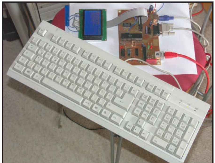
Photo 1—The complete MiniEmail system includes an LCD, a keyboard, and several connections.
