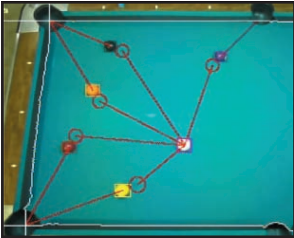
Photo 2 —Here the ghost ball detection is finding five object balls and drawing the expected contact point on each.
