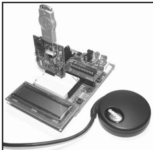
Photo 3 —The first example uses a Cypress PSoc to interconnect a Vinculum chip with a Garmin GPS sensor. The character LCD is used for debugging, but it could be incorporated into the final design.
