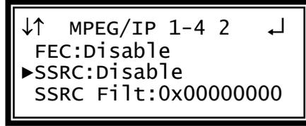
**Synchronized Source Setup Filter**
