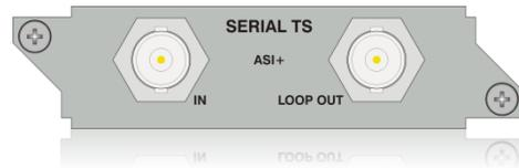
**Description:** This card provides DVB-ASI input for MPTS up to 160 Mb/sec. The maximum TS bitrate for the card is 160 Mb/sec if the stream consists of a MPTS where no program within the stream is greater than 54 Mb/sec. The output on the card is a passive loop-through and should be terminated with a 75 ohm terminator when not in use. The card cannot be used to provide a TS output from another TS input on the unit.
