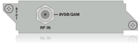
**Description:** This card provides demodulation of 8VSB or QAM. For 8VSB the card is able to tune to channels 2-69 on UHF/VHF and channels 2-134 on the cable channel bands of FCC cable, IRC, and HRC. For QAM, the card is able to receive both QAM64B and QAM256B and is able to tune to channels 2-134 in the cable bands of FCC cable, IRC, and HRC.
