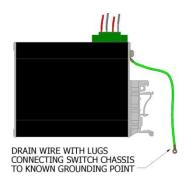
Users may run a drain wire & lug from the screw provided on the back face of the enclosure. In the event the provided grounding screw has been lost, care should be taken to limit the penetration of the outer skin by less than 1/4". Failure to do so may cause irreversible damage to the internal components of the switch.
