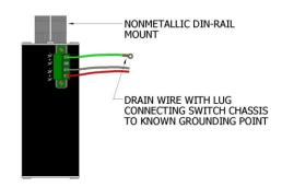
If the use of shielded cables is required, it is generally recommended to only connect the shield at one end to prevent ground loops and interfere with low level signals (i.e. thermocouples, RTD, etc.). Cat5e cables manufactured to EIA-568A or 568B specifications are required for use with N-Tron Switches.
