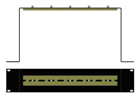
Most N-Tron<sup>TM</sup> products are designed to be mounted on industry standard 35mm DIN rail. However, DIN rail mounting may not be suitable for all applications. Our Universal Rack Mount Kit (P/N: URMK) may be used to mount the 105TX/FX-POE enclosures to standard 19" racks as an option.
