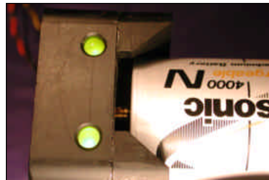
Figure 7-7: Translation Lock Battery Holder
