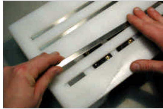
Figure 7-9: Assembling the Power Rails
