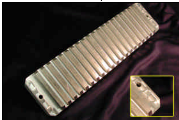
Figure 9-10: External Heat Sink. Inset: Beveled Corner
