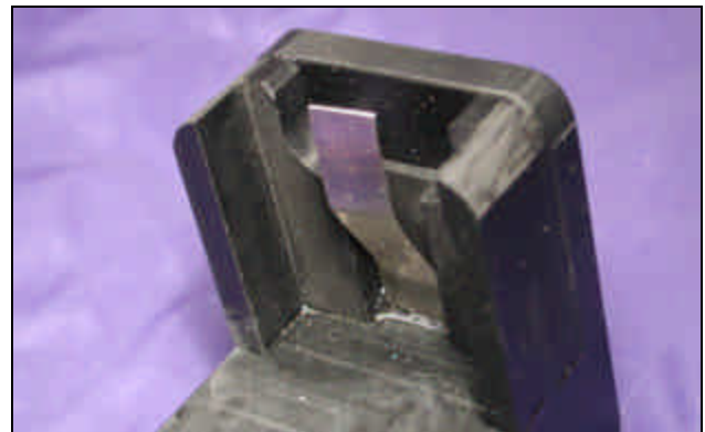
Figure 9-15: Detail of Positive Battery Contact
