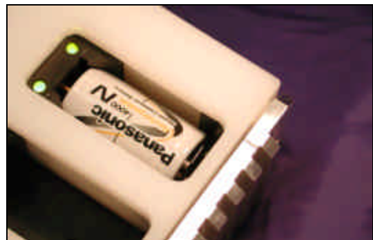
Figure 7-12: Cell Charger Visible Through Access Port
