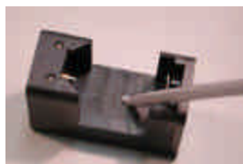
Figure 9-9: Potting Applied to Sensor
