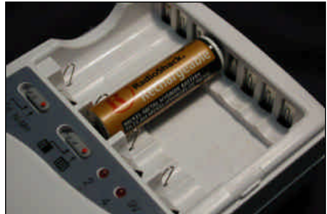
Figure 9-17: Battery Holder in a Consumer Grade Fast-Charger
