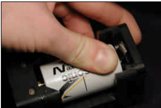
Figure 9-21: Inserting a Battery (Stage 2)
