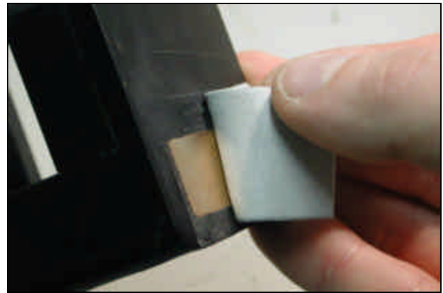
Figure 9-7: Installing a Thermal Interface Pad
