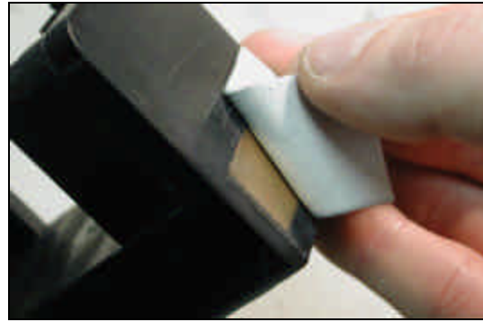
Figure 7-5: Applying a Thermal Interface Pad
