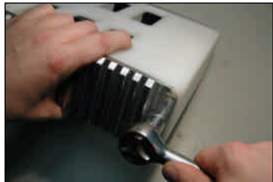
Figure 7-11: Securing the External Heat Sinks
