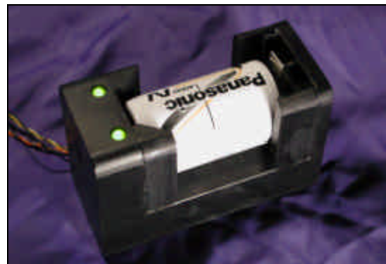
Figure 7-4: Cell Charger Module in Use
