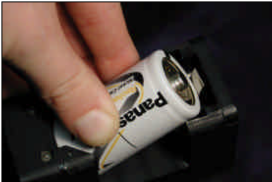
Figure 9-20: Inserting a Battery (Stage 1)
