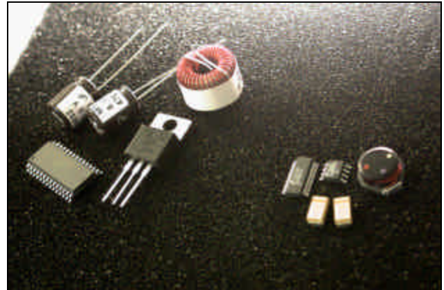
Figure 17-1: Switching Regulator Components
