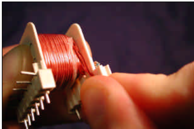
Figure 10-11: Winding the LV Flyback By Hand
