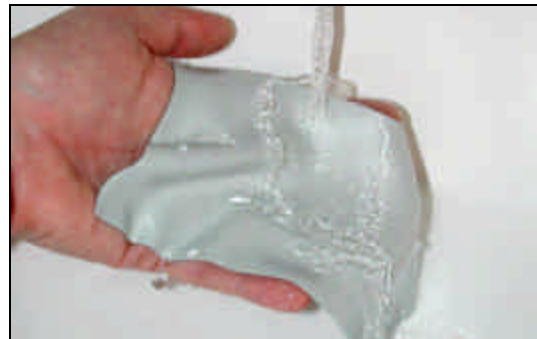
Figure 7-6: Washing a Thermal Interface Pad
