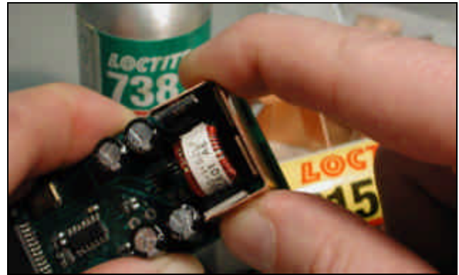
Figure 9-6: Securing the Heat Spreader
