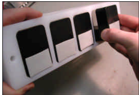
Figure 7-10: Loading Cell Charger Modules Into Chassis
