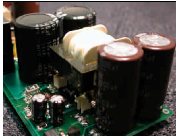
Figure 10-15: Detail of High Voltage Converter
