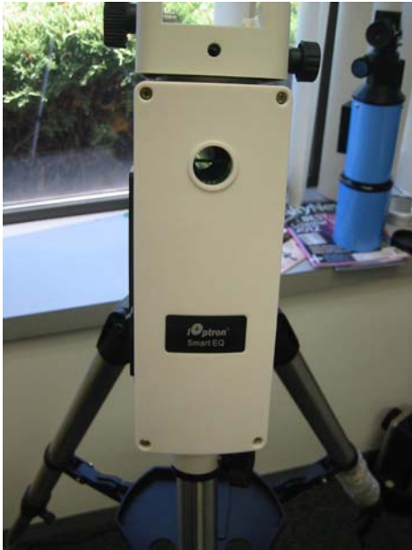
Figure 5. Remove face plate screws
