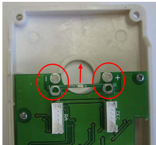
Figure 7. Align LED to the main board
