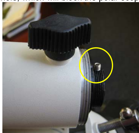
Figure 2. Insert M4 set screw
