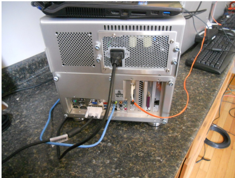
Figure 5: Back panel of Bolt-II computer, showing cables.
