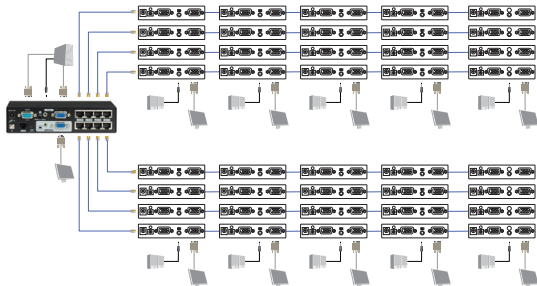
Figure 3-4. Connection pattern for 4-/8-Port Transmitter + Cascadable Receiver + Receiver (Non-Cascaded Application).
